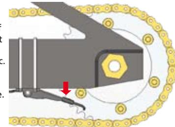
4.) Once happy with the positioning, secure cable ties and trim approx 10 to 12cm from the end of the tail of the Dual Injector. (Keep this to make replacement nibs - see website).
