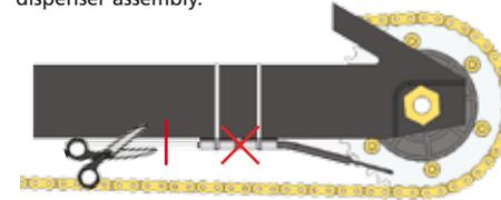
2.) Clean sprocket and chain and hold the Dual Injector Mounting Block (part 2) with bolt (part 1) on the underside of swingarm.
