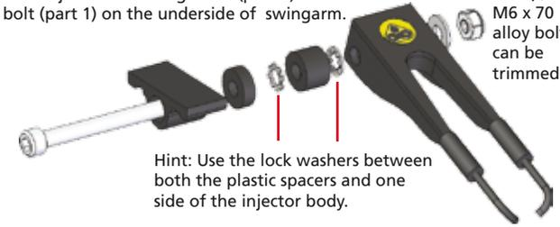
Hint: Use the lock washers between both the plastic spacers and one side of the injector body.
