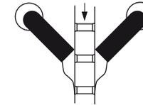
3c.) Keep nibs clear of the sprocket teeth/chain interface etc. Turn wheel to check no interference.
