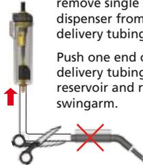
1b.) If updating an existing installation, either vacuum or electronic, trim back the original single sided dispenser to clear tube and remove dispenser assembly.
