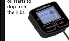
Navigate to the 'Driving Screen'. Use the 'set' button to cycle through the desired flow rates until 60-70 seconds per drop (s/dp) is shown. Check chain condition after a short journey and adjust as necessary.
