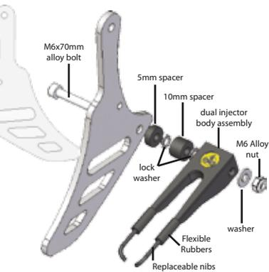
Fit the dual injector body as shown above, referring to Steps 3a,b,c in Set-Up Guide.
