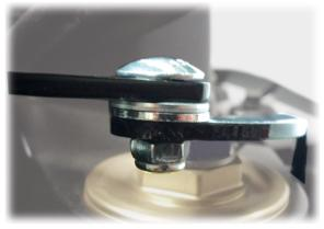
Mount the windshield/screen on the bracket (picture 1). Remove the fixing screws of streering plate, insert the thickness high 13 into the screw position, approach the "B" stirrup and insert the 8x45 screw (picture 2). Don't lock. Mount the windshield/screen with the bracket mounted before on the "b" stirrup using the "squadre shape" screw diameter 6, the washers and the autolock nut (picture 3). Find ideal position of windshield/screen and than fix all the the screws
