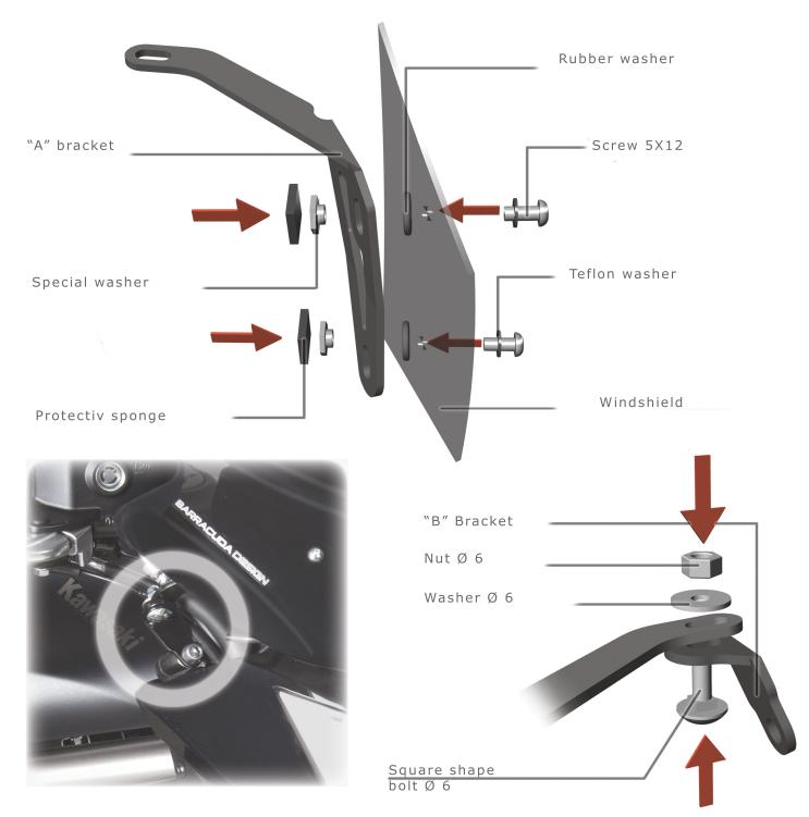
ASSEMBL THE BARRACUDA WINDSHIELD/SCREEN USING THE SCREWS AND THICKNESS INCLUDED IN THE KIT. MOUNT ALL LIKE THE INSTRUCTION, AT THE END UNLOCK THE FORK UPPER SCREWS AND SUSTITUTE THEM WITH THE 8X50 SCREWS TOGHETER WITH THE HIGH 10 THICKNESS. WE ADVICE TO LOCK ALL TOGHETER ONCE YOU FIX THE WINDHSIELD/SCREEN TO AVOID BROKEN PART DUE TOO FORCING
