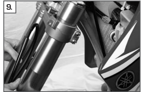
9. Pull the fork down and remove together with the front wheel and brake system.
