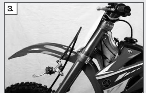
Attach the brake pump to the brake line.
