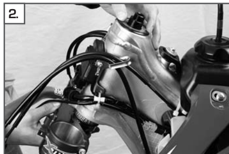
2. Slide the lower triple clamp into the steering head, holding the upper steering head bearing and the sealing washer in place.
