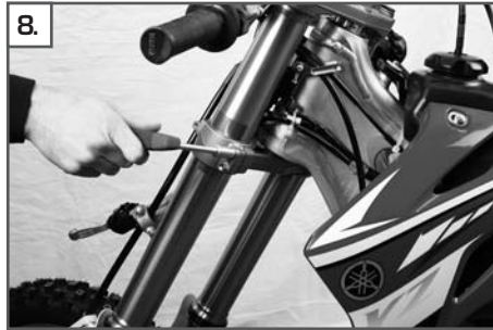
8. Loosen the triple clamp clampings.
