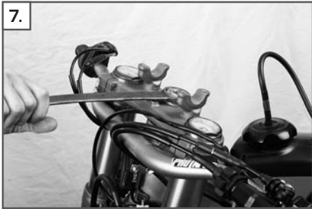
7. Loosen the mounting nut on the upper triple clamp.
