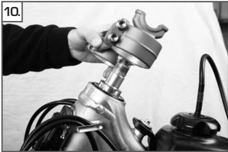
10. Remove the upper triple clamp.
