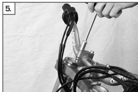
Remove the handlebar and any fastening material such as cable ties.
