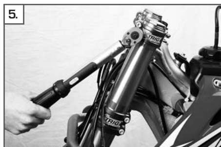
5. Position the fork, front wheel and brake system in the triple clamp.
