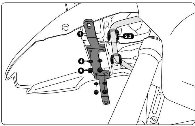
**Step One:** Position the two U-Bolts onto the subframe just behind the oil cooler. The smaller U-Bolts (#2) are for use with the standard R1200GS, the larger (#3), are for use with the R1200GS Adventure.
