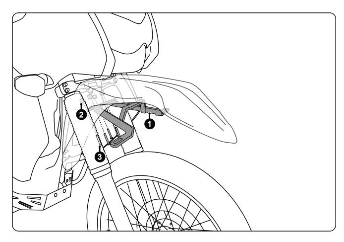
**Step One:** Remove the four bolts on the underside of the front fender. Using the supplied hardware mount the light bracket to the motorcycle as illustrated above.
